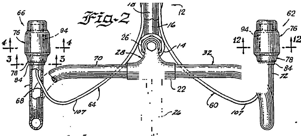
As depicted above in Figure 2, the shift actuators are mounted over the ends of a traditional drop bar-type handlebar 32. *Id.*, col. 9, ll. 31-33. The handlebar 32 has “generally straight rearwardly directed end portions 72 over which handgrip shift actuators 62 and 66 of the invention are mounted.” *Id.*, col. 9, ll. 41-46. During cycling,
