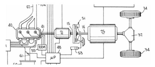
Consequently, when the clutch is disengaged, the electric motor is the sole source of torque transferred to the wheels. When the clutch is engaged, however, torque provided by both the ICE and the electric motor is transferred to the wheels. Another
