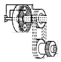
See J.A. 1256,<sup>5</sup> 12788. In particular, Dr. Nichols stated that the structure is (1) "a multi-input device or component"—it accepts inputs at the planetary carrier from the ICE output shaft and at the ring gear from the MG2 output shaft; (2) "that is controlled to transfer variable amounts of torque"—the microprocessor dictates the amount of torque sent from each input, and ultimately output to the drive shaft. See, e.g., J.A. 1201-03.
