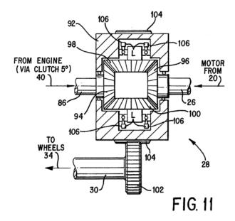
As shown in figure 11 of the '970 patent, illustrated above, the ICE output shaft 86 and the electric motor output shaft 26 extend into the CTTU housing 92 and terminate at bevel gears 94 and 96, respectively, each of which mesh with two other bevel gears, 98 and 100.
