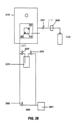
This embodiment mounts a hybridization chip package on vortexer 2910. Container 2930 then fills with fluid containing targets. At that point, various valves open to allow nitrogen gas from 2901 to enter container 2930, thereby forcing fluid into the cavity 310.
