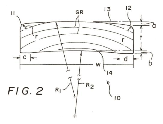
As shown, the top of the board is in a convex shape so that water will flow from its middle to its sides. Correspondingly, the bottom of the board is concave so that other boards can be stacked below it. Claim 1 contains all pertinent terms and is representative of the asserted claims:
