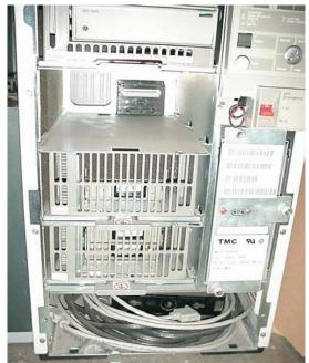
IBM AS/400 System with Drive Bays Exposed
