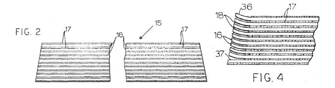
As shown in the figures above, pad 15 consists of a plurality of plastic sheets 16 with acrylic latex adhesive layers 17 above and below each of them. The adhesive layer beneath the lowermost plastic sheet releasably attaches the sheet—along with the rest of the pad—to the top surface of the floor. See id. at col.4 II.49-51 ("The lowermost sheet 16 has on its undersurface 22 a layer 23 of adhesive to removably affix the pad 15 to the floor 14.").
