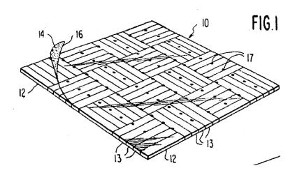
A plastic cover sheet 16 is attached to a set of floor tiles 12 using an adhesive 14. "[P]lastic cover sheet 16 . . . is formed from a transparent or translucent plastic film . . . e.g., four mil low density polyethylene film." <u>Id.</u> at col.6 II.2-8.
