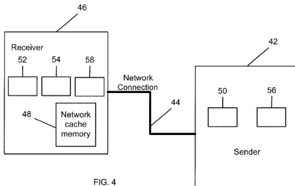
In this embodiment, the receiver/computer (46) sends a request for data to the sender/computer (42). The sender/computer calculates a digital digest on the data stored in its memory and transmits the digest to the receiver/computer. The receiver/computer then searches its
