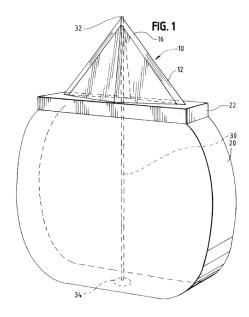
The Samuels scalpel possesses a central lumen 30, which extends through the length of the blade 10, the blocker 22, and the handle 20. Samuels teaches that the "blade is . . . advanced into the patient's skin until [the] blocker impedes further travel. As such, [the] blocker limits the depth of the skin nick formed." Samuels, col. 4 ll. 54–57 (citations to figure omitted).
