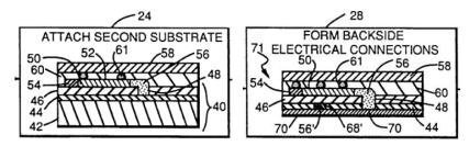
*Id.* fig.1. (boxes 24, 28). Once the wafer and circuitry are supported, the back side of the first substrate is removed. *Id.* col. 5, ll. 45–51. Finally, as shown in box 28 of Figure 1, various back-side electrical connections are formed through the remaining portion of the first substrate. *Id.* col. 6, ll. 10–15, 44–49.
