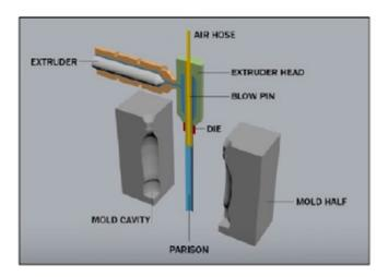
J.A. 3482 (Appellee's Technology Tutorial). The image shows the general placement and geometry of the extruder head, die, parison, and molding cavity in a conventional blow molding process.
