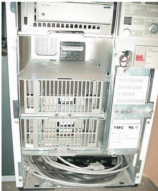
IBM AS/400 System with Drive Bays Exposed
