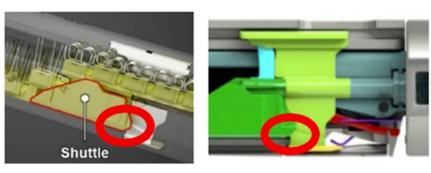
Appellant's Reply Br. 37 ("[T]he protrusion on the beam's lower portion contacts the shuttle as indicated by the red circles, which correspond to where [Rex's technical expert Albert Juergens III] pointed with his laser pointer during
